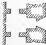
HORIZONTAL SECTION THROUGH CASEMENT
